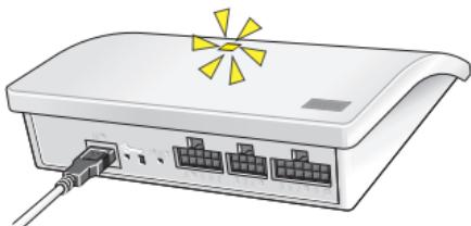
When the light-emitting diode flashes yellow, the interface has been reset. This may take up to 1 minute.
