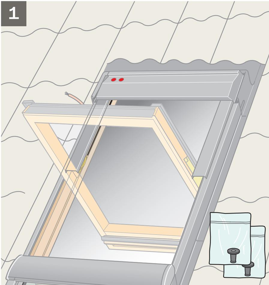
**ENGLISH:** If the window has been fitted with a black screen profile and/or a connection box, remove this/these temporarily **[a]**, **[b]**. Drill hole **[c]** and fit rubber grommet **[d]**. Pull grommet through from the inside **[e]**.
