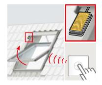
The window can be opened again with the wall switch when the rain sensor is dry.
