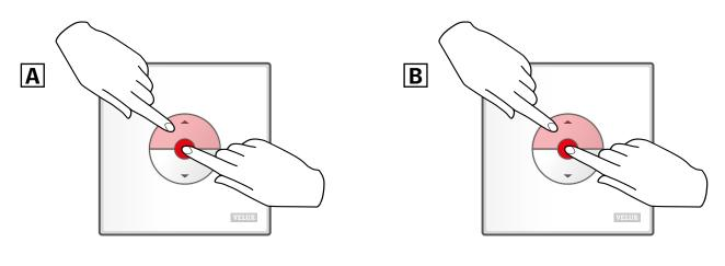
Press OPEN/UP and STOP key simultaneously for **more** than 1 second.
