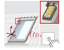
The rain sensor prevents the roof window from opening for as long as it detects rain.
