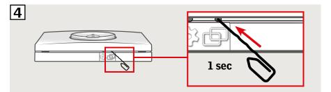
Press the STOP key and then the DOWN key within 3 seconds.
