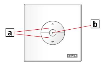
Wall switch KLI has two buttons used for setup:
