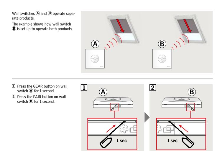
Wall switch (B) can now operate both products. Wall switch (A) can still operate its own product.
