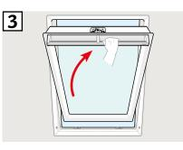
When the window has been closed with the control bar, it will automatically close completely.
