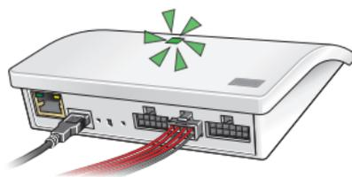
Short-circuit wires (1 second) in the double input which is to control the chosen product(s). It can take up to 1 minute before the light-emitting diode flashes green and the product(s) is/are assigned to the input terminal on the interface.
