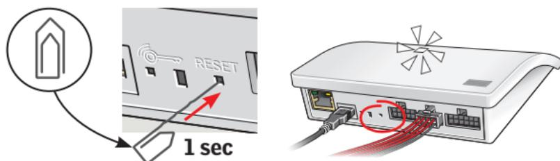
Connect the supplied wire bundle to the input terminal. Press the RESET button on the back of the interface briefly (1 second) with a pointed object. The light-emitting diode flashes white rapidly. Step 15 must now be carried out within 2 minutes.
