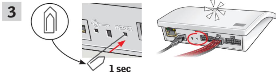
Press the RESET button on the back of the interface briefly (1 second) with a pointed object. The light-emitting diode flashes white. Step 4 must now be carried out within 2 minutes.
