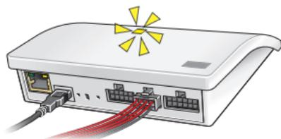
Connect the interface to the mains supply and connect the supplied wire bundle to the input terminal. When the light-emitting diode flashes yellow, the interface is ready for configuration.
