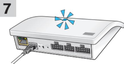
When the blue light-emitting diode is on, the interface is configured as a repeater.
