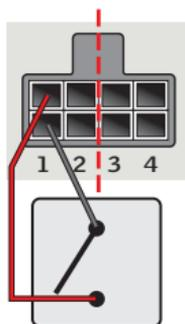
A set of two contacts can be used for running products both up and down with variable stops by pressing both contacts simultaneously.
