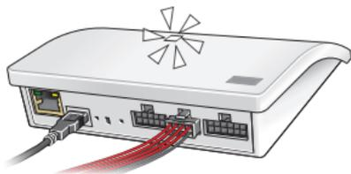
When the white light-emitting diode is on, interface KLF 200 has been configured as an interface.
