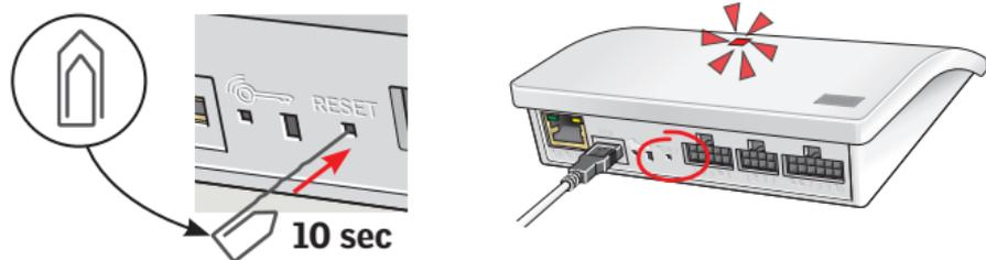
Press the RESET button on the back of the interface for 10 seconds with a pointed object until the red light-emitting diode is on. After this, the light-emitting diode will turn yellow followed by a red flash.
