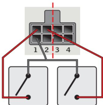
A change-over contact can also be used for running products both up and down but stops are not possible, for instance for a thermostat.
