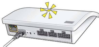
Connect the interface to the mains supply. When the light-emitting diode flashes yellow, the interface is ready to be configured.
