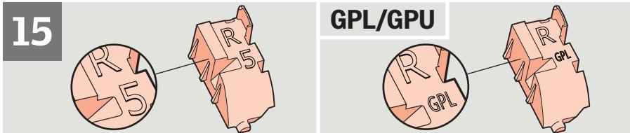
**ENGLISH:** Fit plastic insert pieces on the roller shutter side channels **a**, **b**.
