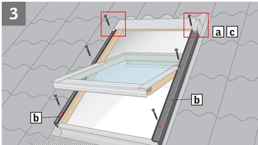
**ENGLISH:** Remove cover screws except the top cover screw **a**. The number of screws depends on the size and type of the window. Do **not** remove side frame covers **b**. If there is a mark at the top instead of a hole, drill hole through mark **c**. Place sealant on **all** screw holes **d**.
