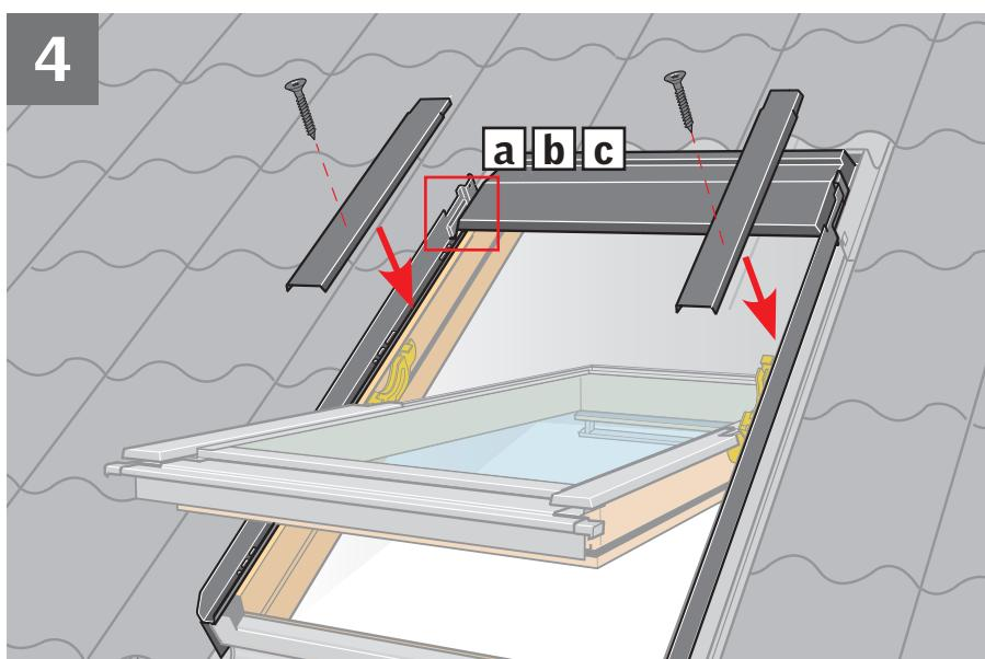
**ENGLISH:** Loosen screws in top cover **a**, **b** or **c**. Fit window covers using existing screws. Re-tighten top cover screws.
