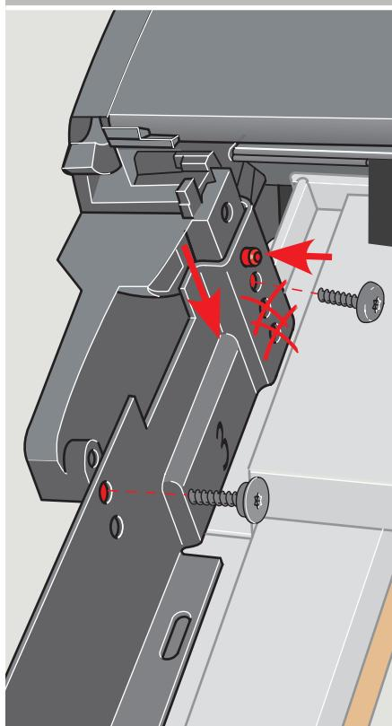
**ENGLISH:** Lower the roller shutter top casing as much as possible. Do **not** press the top casing against the roofing material **[a], [b]**. Fit securing screws after installing the roller shutter top casing **[c], [d]**.
