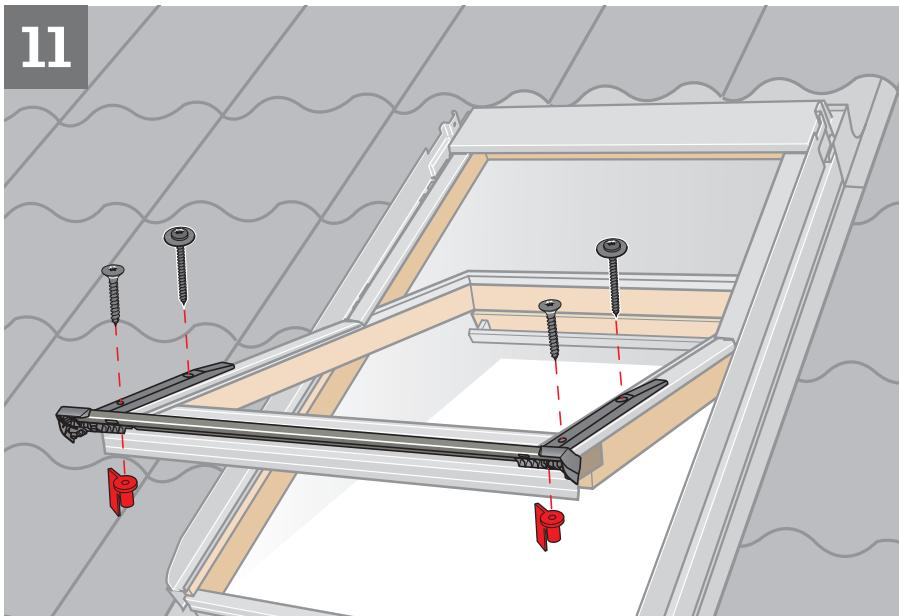
**ENGLISH:** Fit bottom cover. Secure lower screws with special nuts.
