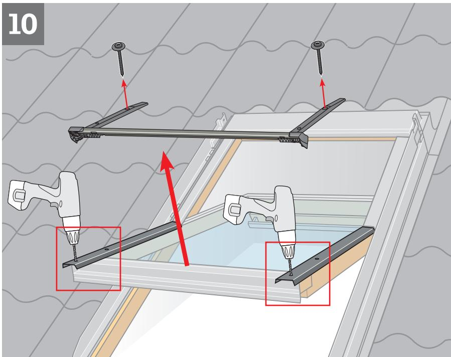
**ENGLISH:** Remove bottom cover temporarily and drill lower holes **a**. Place sealant on **all** screw holes **b**.
