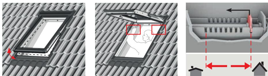
**ENGLISH:** The sash should be able to remain open in any position; otherwise, springs must be adjusted as shown.
