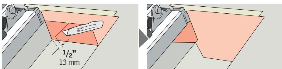
**ENGLISH:** To allow for proper drainage, interweave VELUX adhesive skylight underlayment as shown in **6a** for new construction applications. For retrofit applications, interweave VELUX adhesive skylight underlayment as shown in **6b**.
