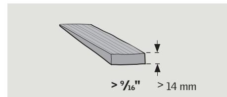
**ENGLISH:** EDL cannot be used for cedar shingles and slates thicker than 5/16" (14 mm). In this case, see installation instructions for flashing EDW (for profiled roofing materials).
