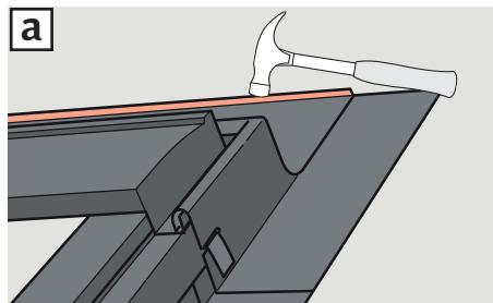
**ENGLISH:** To allow for proper drainage, interweave roofing underlayment as shown.
