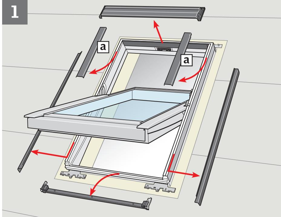
**ENGLISH:** Remove cladding as shown to allow for proper installation of underlayment.
