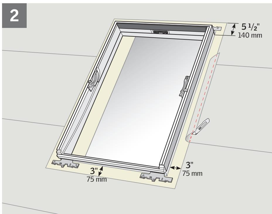
**ENGLISH:** Remove existing roofing underlayment around the rough opening as shown.
