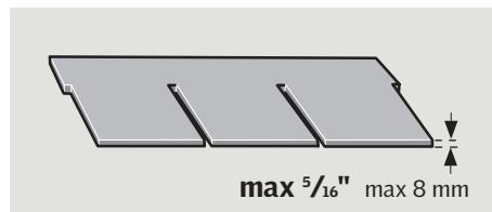
**ENGLISH:** EDL is designed for thin roofing materials (max thickness 5/16" (8 mm)).
