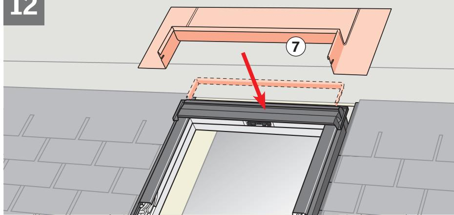
**ENGLISH:** Install saddle flashing. Determine use of extension piece: use it if the saddle flashing is lifted up by the underlying roofing material and remove it if the saddle flashing fits tightly over the window.
