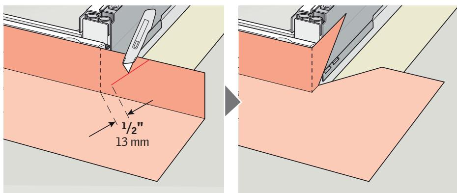
**ENGLISH:** To ensure waterproofing, window frames should be completely wrapped in underlayment. Your VELUX sales company recommends using VELUX ZOZ 216 adhesive skylight underlayment. This underlayment must be applied before installing the flashing.
