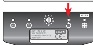
A ventilation filter can last about 4000 operating hours. When the filter is to be replaced, the yellow light-emitting diode is on.
