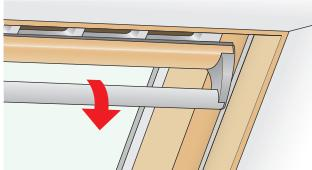
When you open the ventilation flap of the roof window, you automatically switch on the built-in ventilation system. When you close the ventilation flap, you switch off the ventilation system.
