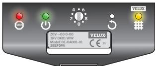
When connecting the heat recovery ventilation unit to the 230 V mains supply, all three light-emitting diodes are on for 2 seconds to indicate correct connection.
