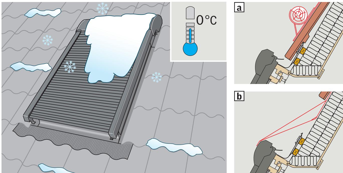
**ENGLISH:** As a precondition to avoiding any damage to the roller shutter in very cold regions and in regions with heavy snowfall, either a snow-wedge or a snow stop must be installed above the roller shutter **a**, **b**. In case of snow on the roof, care must be taken when operating the roller shutter.
