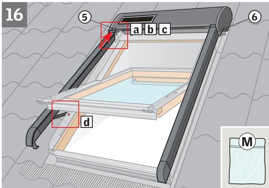
**ENGLISH:** Fit side profiles **a**. Insert and fix pins for hinges **b**, **c**. Attach opening restrictors to side covers with screws **d**. The roller shutter is now ready for use. For important information, see pages 24-26. For operation of the roller shutter, see enclosed directions for use.
