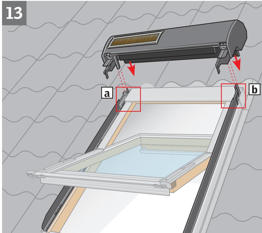
**ENGLISH:** Fit roller shutter top casing into grooves on side covers **a**. Check that rubber gasket at the back fits smoothly against outside of window **b**.
