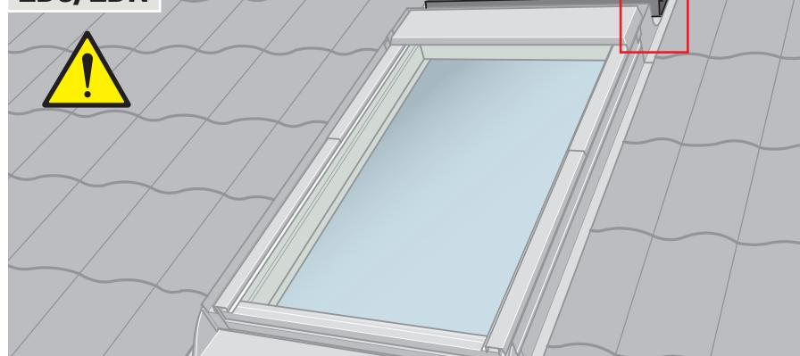
**ENGLISH:** If roller shutter is to be installed with flashing EDJ or EDN: Bend down rainwater deflector to make room for roller shutter.
