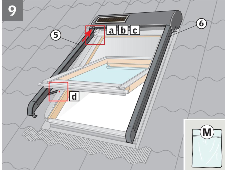
**ENGLISH:** Fit side profiles **a**. Insert and fix pins for hinges **b, c**. Attach opening restrictors to side covers with screws **d**. **The roller shutter is now ready for use. For important information, see pages 24-26. For operation of the roller shutter, see enclosed directions for use.**
