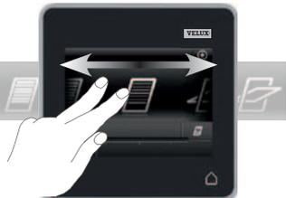
You operate all products by tapping icons/buttons or by dragging the slider and tapping the bar in the display.
