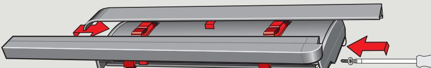
**ENGLISH:** Remove plastic covers from both sides **a**. Place adapter on axle and turn into position **b**. Fix adapter with screw supplied **c**. Refit plastic covers **d**.
