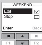
6 To interrupt the program VELUX ACTIVE for a given period of time, the starting and end time must be set.
