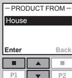
4 Displays a list of all products in House. The product type, in this case skylights (indicated as "Window"), appears in the display. The individual products can be identified by pressing **Hold** for a short period of time. This will activate the product briefly.
