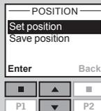
6 Press to set the opening position of the skylight. 100% corresponds to fully open. Press "Enter" to confirm your setting.
