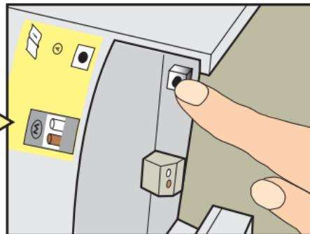
**English:** Control system KUX 100 can be reset by removing the control unit cover and pressing the test button for 10 seconds.
