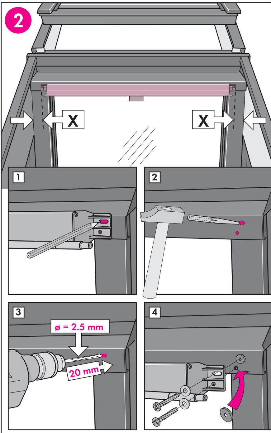
**ENGLISH:** Place awning blind in the centre of the window as shown. Mark holes on both sides of the awning blind with a pencil (1). Start holes with a centre punch (2) and drill through the cover using 2.5 mm drill. Drilling depth = 20 mm (3). Place sealant supplied on exterior of covers. Fix awning blind with screws and washers supplied (4).
