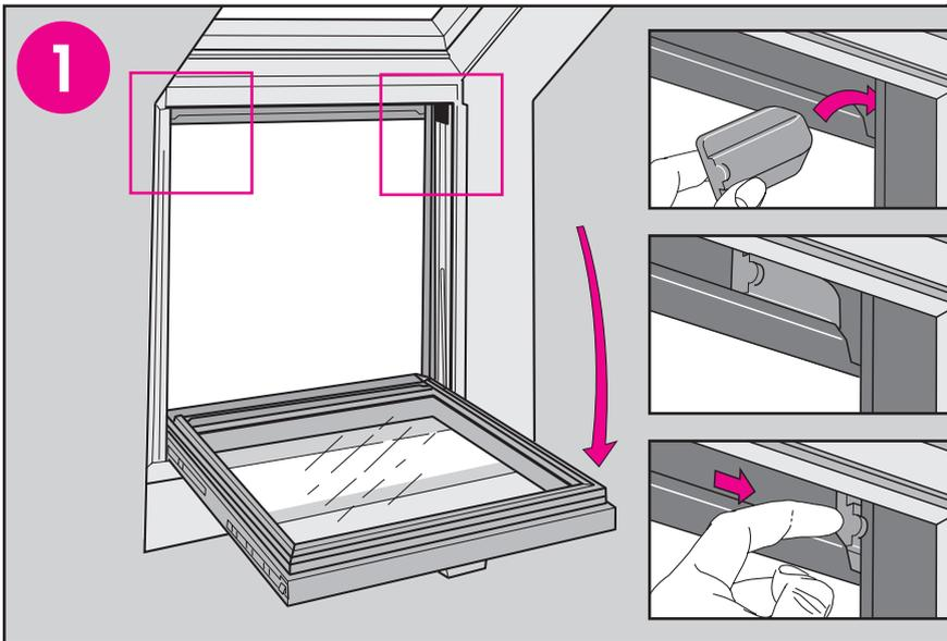
**ENGLISH:** The sash may be removed to simplify installation (see page 4). Fit plastic pieces with flat side against top cover in the top corners as shown.
