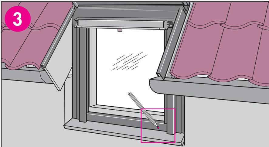
**ENGLISH:** Fix hooks on the external horizontal window cover as shown. Mark holes with a pencil (1). Start holes with a centre punch (2) and drill through the cover using a 2.5 mm drill. Drilling depth = 30 mm (3). Fit hooks with screws (4).
