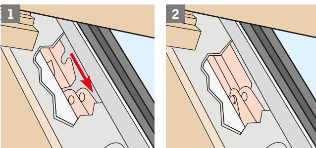
**ENGLISH:** **Connection of springs with fittings:** Push sash upwards, ensuring that fittings and springs on both sides automatically connect **1 , 2 .**
