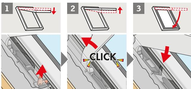
**ENGLISH:** **Disengage springs:** Open window sash completely and pull slightly downwards. Then lift coupling plate as shown **1**. Push sash upwards to disengage the springs **2**. Close sash **3**.
