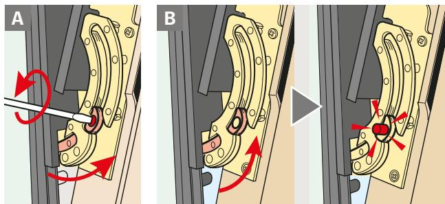
**ENGLISH:** Replace window sash: The push button is automatically released, when the window is closed **A** , **B** .
