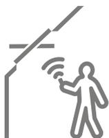
VELUX INTEGRA® remote-controlled roof windows are easily operated by a wireless wall switch, providing fresh air at the touch of a button. Perfect for both within-reach and out-of-reach applications where extra comfort and convenient operation is required. Available in mains- and solar-powered versions. For optimum daylight, choose larger windows for lower roof pitches.
