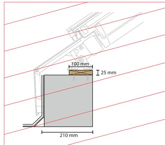
Steel, concrete or wood construction with wooden batten
