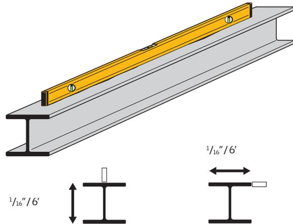
The following standard steel profiles are suited for installation of VELUX modular skylights in Step Longlight solutions.
