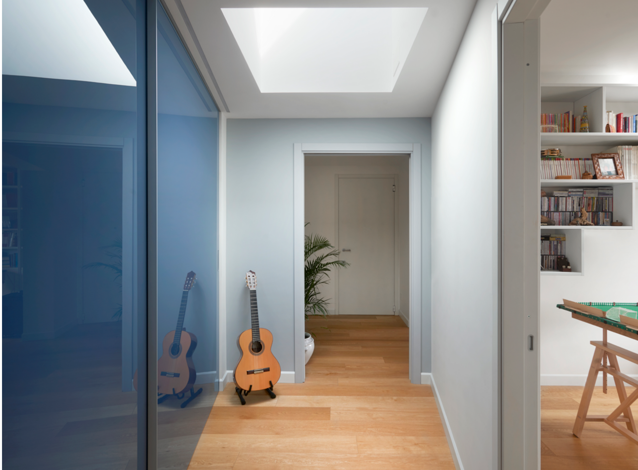
Corridor Daylight need for corridors is 100 lux, which corresponds approximately to 1% Daylight Factor
