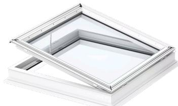
Enjoy ultimate convenience and remote-controlled ventilation with an electric base unit CVP QA. A burglary-resistant construction with P4A laminated inner glass delivers maximum security, while the insulated ThermoTechnology™ PVC construction and low-energy glazing with two energy coatings help keep your home warm and energy costs low. Compatible with all VELUX flat-roof window ISD top units.
