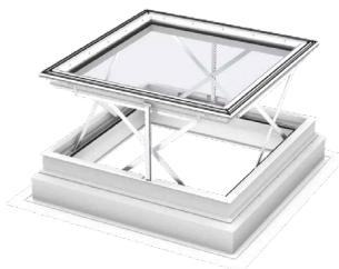
The flat-roof smoke ventilation window CSP will automatically open in case of fire and meets all relevant EU legislative requirements. The window can be opened for fresh air when ventilation is needed. A burglar-proof construction provides additional security and a laminated inner pane prevents glass from splintering in the event of breakage.
