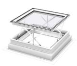
The flat-roof smoke ventilation window CSP will automatically open in case of fire and meets all relevant EU legislative requirements. The window can be opened for fresh air when ventilation is needed. A burglar-proof construction provides additional security and a laminated inner pane prevents glass from splintering in the event of breakage.
