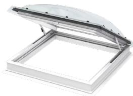
The manually operated flat-roof exit window CXP opens extra wide to provide easy access to the roof. A laminated inner pane prevents glass from splintering in the event of breakage. Available with an acrylic and polycarbonate dome. The flat-roof exit window meets all relevant EU legislative requirements.
