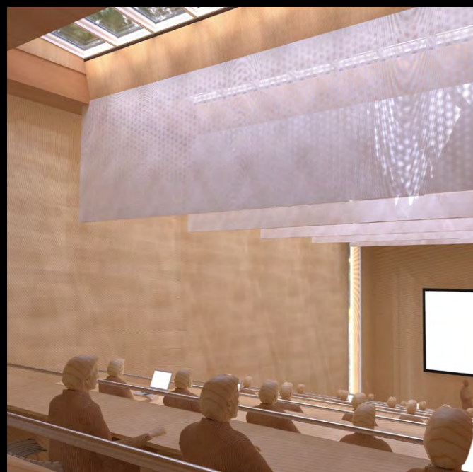
Scenario 5: Blocking and reflective vertical inside panels
