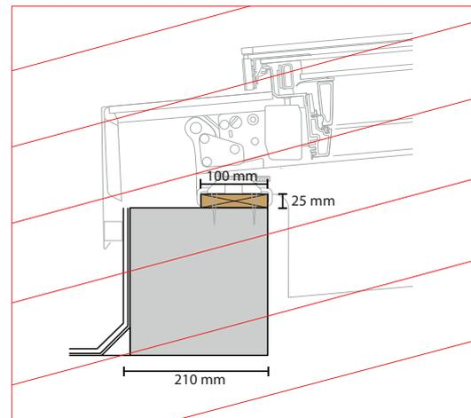
Steel, concrete or wood construction with wooden batten
