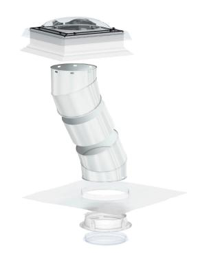
Get the most natural daylight out of your VELUX sun tunnel with the rigid tunnel. The rigid tunnel has a super high reflective coating that delivers up to 98 % daylight reflectivity for optimum natural light conditions in your home, even on cloudy days. Recommended for lengths between 0.9 and 1.7 m and is effective up to 6.0 m using tunnel extensions.
