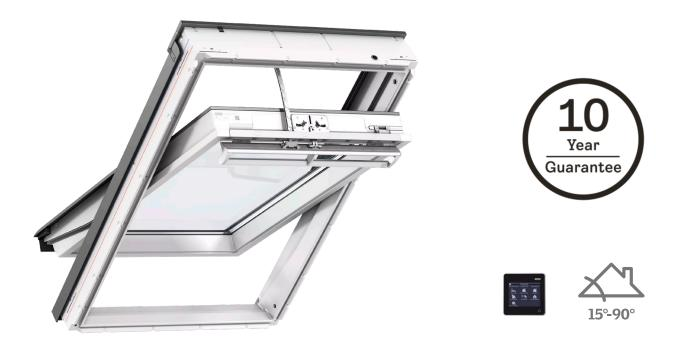
The VELUX electric, centre-pivot roof window GGU is a wired solution that operates remotely using a control pad – perfect for both in- and out-of-reach installations. The roof window has an integrated motor and a rain sensor that automatically closes the window if it rains. Moisture-resistance makes it ideal for kitchens and bathrooms.
