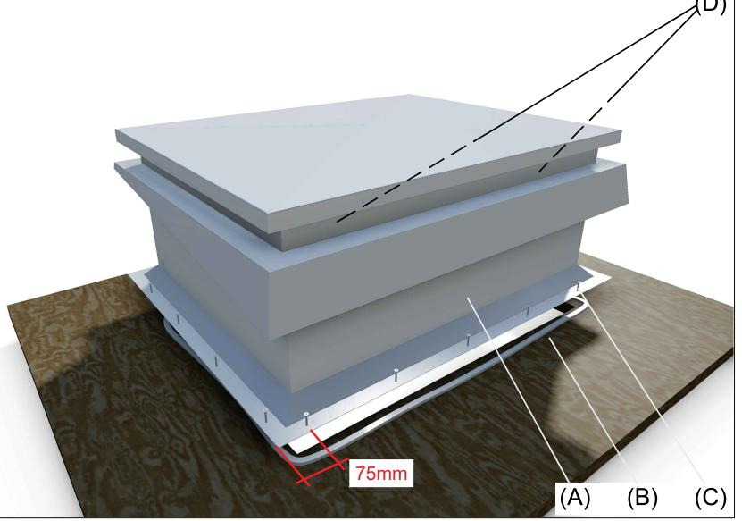
NOTE:- Contractor is to provide a flat level surface minimum 100mm around the roof opening. Sealant and fasteners at roof deck level not by Xtralite
