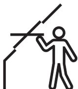
Manually top-operated, centre-pivot roof windows make it possible to place furniture directly below the window without obstructing the window's operation. We recommend an installation height that allows for a clear sight line to the outside from both a standing and seated position. Please note that the optimum window height depends on the roof pitch.
