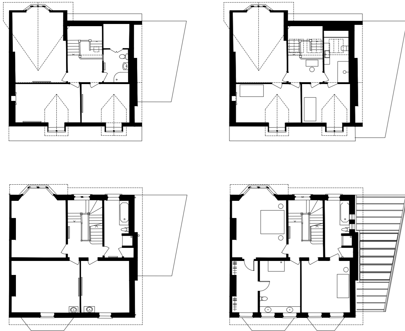
Above: Top floor, before and after the refurbishment. What used to be a gloomy and stuffy bathroom has become a light-filled, well ventilated shower room for the boys. Two VELUX Heritage Conservation windows bring daylight deep into the house. The homeowners have plenty of ideas about how to enhance the space further. Below: First floor, before and after the refurbishment. Carly and Andrew decided to sacrifice one bedroom to create a bright shower room and an en-suite dressing room. The additional windows on the garden facade, as designed by Spence & Dower for the planning application, will further enhance the rooms in the future.
