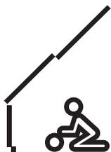
The vertical window element VIU is installed vertically directly below a VELUX roof window. As it stretches nearly to the floor, it provides more daylight and an enhanced view when standing and when seated. The vertical window element VIU is fixed and cannot be opened.
