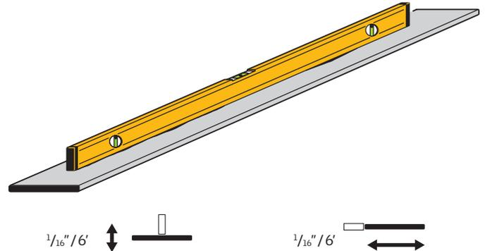
The following standard flat steel profiles are suited for installation of VELUX modular skylights in Longlight solutions.
