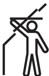
Manual bottom-operated, centre-pivot roof windows are our recommended solution when the window needs to be placed in a high position (130-160 cm) above floor level, for instance because of a high knee wall. In installations in combination with façade elements or as the lower part of a combi installation, bottom operation will be comfortable, as the handle will be easy to reach for opening and closing the window.
