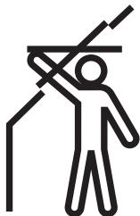
Manual bottom-operated, centre-pivot roof windows are our recommended solution when the bottom of the window is between 130-150 cm over the floor because of a high knee wall. Try to ensure a minimum top level of the window of 200 cm to allow for a clear view to the outside. Please note that the optimum window height depends on the roof pitch.
