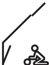
The vertical window element VFE is installed vertically directly below a VELUX roof window. As it stretches nearly to the floor, it provides more daylight and an enhanced view when standing and when seated. The vertical window element VFE opens/tilts inwards and can be secured in ventilation position.
