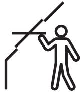
Manually top-operated, centre-pivot roof windows make it possible to place furniture directly below the window without obstructing the window's operation. We recommend an installation height that allows for a clear sight line to the outside from both a standing and seated position. Please note that the optimum window height depends on the roof pitch.
