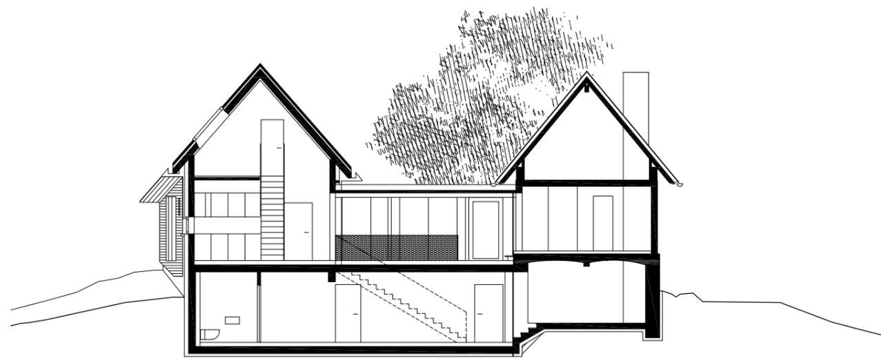
Cross section showing the new house, glazed connecting wing and the old wine cellar building. What is an underground level on the northern edge, is emerging from the hill on the opposite side of the building. At the southern facade, just next to sanitary facilities there is sauna, opening towards a little terrace.
