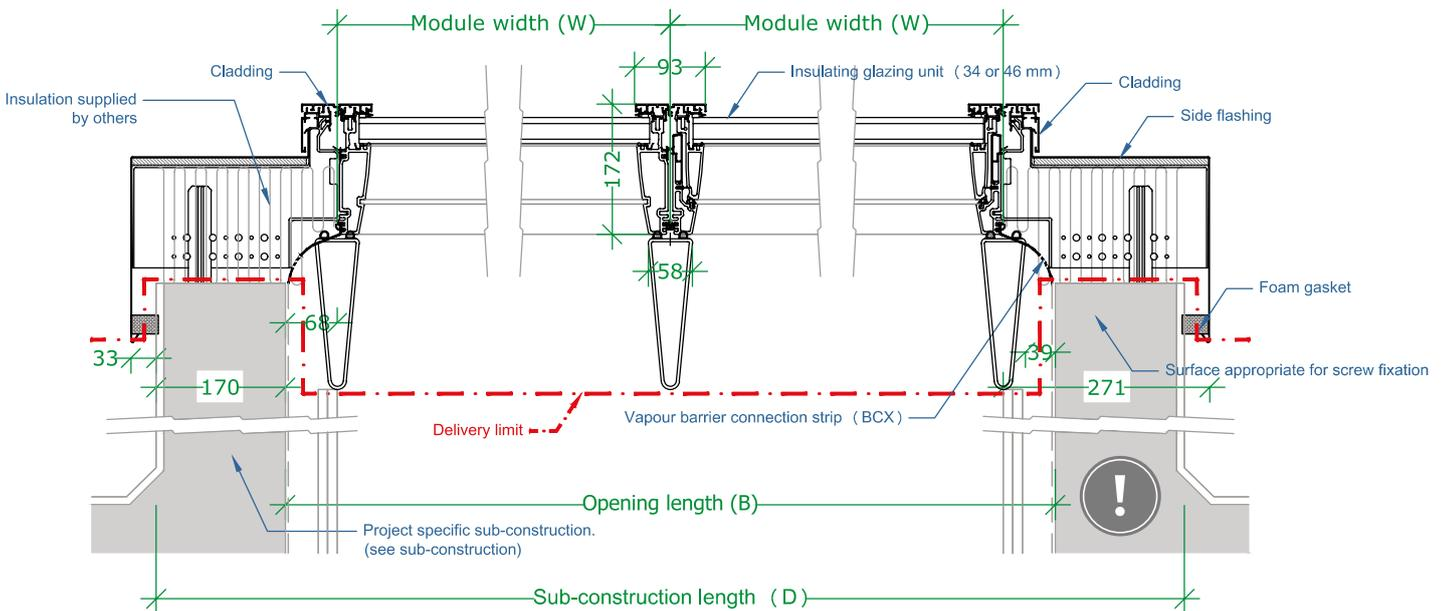
Please observe that a lateral slope on the modules is NOT possible, therefore top and bottom sub-construction must be horizontal.
