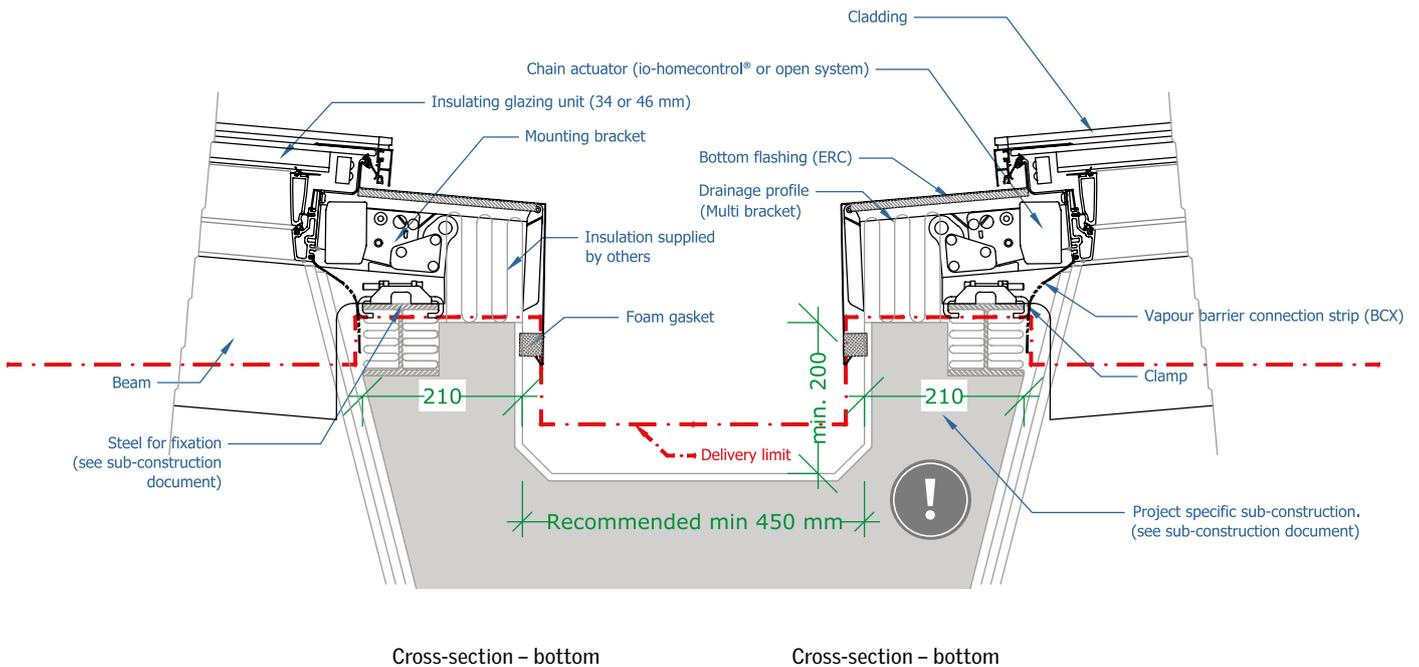
Please observe that a lateral slope on the modules is NOT possible, therefore top and bottom sub-construction must be horizontal.
