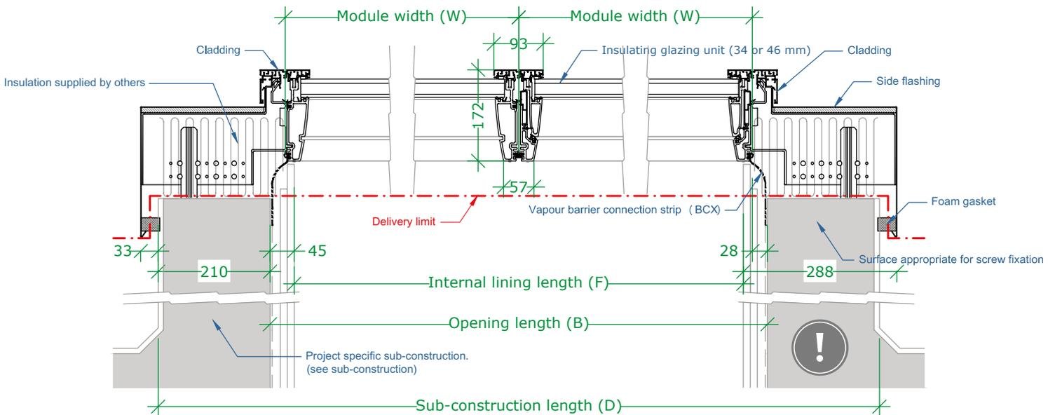
Please observe that a lateral slope on the modules is NOT possible, therefore top and bottom sub-construction must be horizontal.
