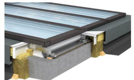
Concrete provides a strong, but heavy sub-construction and is mostly suited for concrete buildings. Concrete sub-constructions are usually cast on site.
