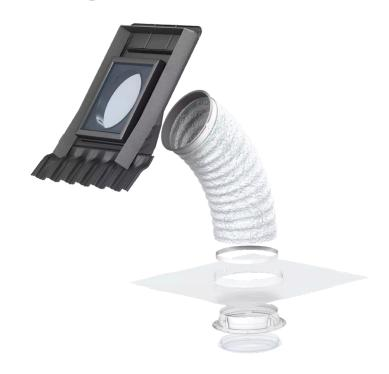
The VELUX sun tunnel with flexible tunnel for pitched roofs TWF is the perfect choice for sun tunnel installations when rigid tunnels cannot be used – i.e. when there is a beam or other obstacle between the roof and the ceiling. Recommended for lengths between 0.4 m and 2 m.
