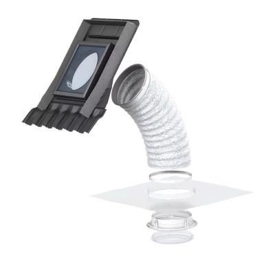
The VELUX sun tunnel with flexible tunnel for pitched roofs TWF is the perfect choice for sun tunnel installations when rigid tunnels cannot be used - i.e. when there is a beam or other obstacle between the roof and the ceiling. Recommended for lengths between 0.4 m and 2 m.
