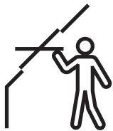
Manually top-operated, centre-pivot roof windows make it possible to place furniture directly below the window without obstructing the window operation. We recommend an installation height that allows for a clear view to the outside from both a standing and seated position. Please note that the optimum window height depends on the roof pitch.
