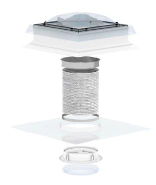
The VELUX sun tunnel for flat roof with flexible tunnel is the perfect choice for VELUX sun tunnel installations when rigid tunnels cannot be used - i.e. when there is a beam or other obstacle between the roof and the ceiling. Recommended for lengths between 0.4 m and 1.5 m for pitched roofs and 0.2 m and 0.9 m for flat roofs.
