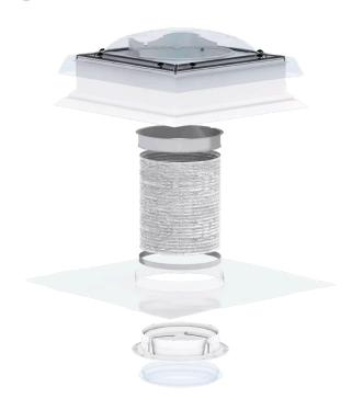
The VELUX sun tunnel for flat roof with flexible tunnel TCF is the perfect choice for VELUX sun tunnel installations when rigid tunnels cannot be used – i.e. when there is a beam or other obstacle between the roof and the ceiling. Recommended for lengths 0.2 m and 0.9 m for flat roofs.
