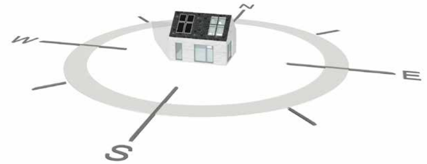
Figure 5.9 Solar energy gain depends on the orientation and slope of the panels.
