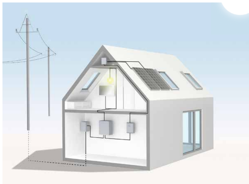
Figure 5.12 Diagram of a solar cell system for private house application.
