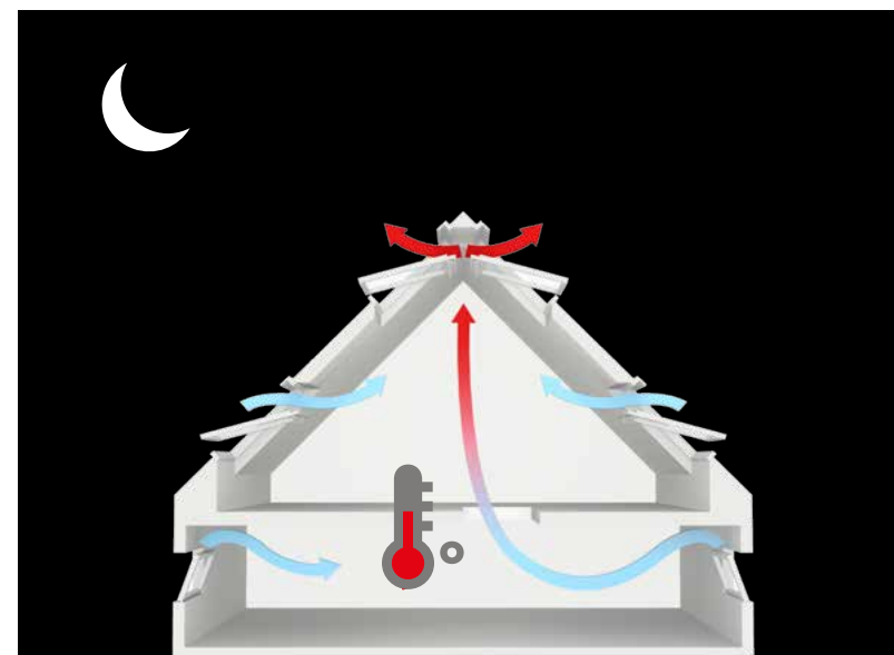
Figure 3.7 – Passive cooling at night (night cooling)
