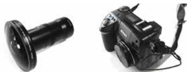
Figure 1.50. Cool pix camera and fisheye lens used to create luminance maps.
