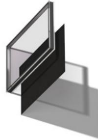
**GLAZING WITH LOW EMISSIVITY COATING AND ROLLER BLIND**
