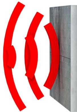
Enclosure in metal. Loss: 90 to 100%
